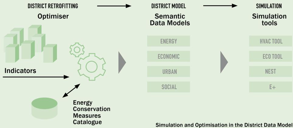
The DDM is populated following a set of data transformation and integration processes based on Semantic Web technologies. This makes the transformation processes transparent and enables the community to maintain them and create new ones. The transformation and integration processes take into account the semantic and structural heterogeneity between the data sources making the DDM an interoperability solution for the architecture, engineering and construction (AEC) industry.
