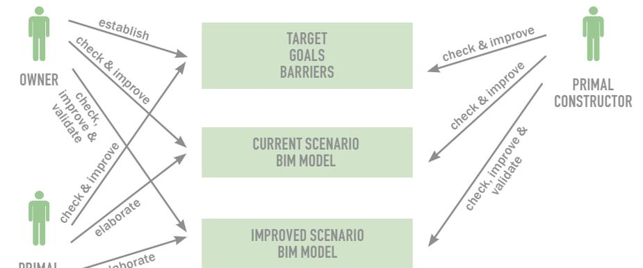
Integrated Approach Process Use Case Diagram (UML notation)
