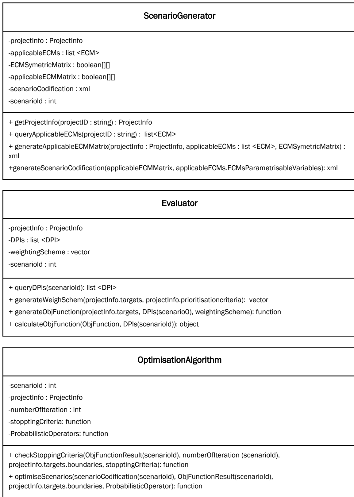
Figure 13: Class diagram of the Optimisation Module
